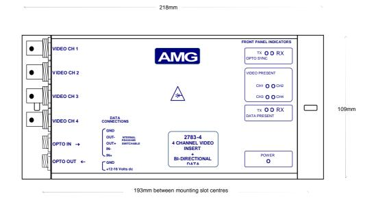
The **AMG2783-4** is a standalone four channel video insert unit designed to transmit four video signals on to a single optical fibre ring. It also provides a RS485/RS422 bi-directional data channel. It is designed to be powered from an **AMG2002** power supply. Up to 8 video channels can be attached to the same single fibre optic ring to transmit up to 8 real time high quality video signals.
